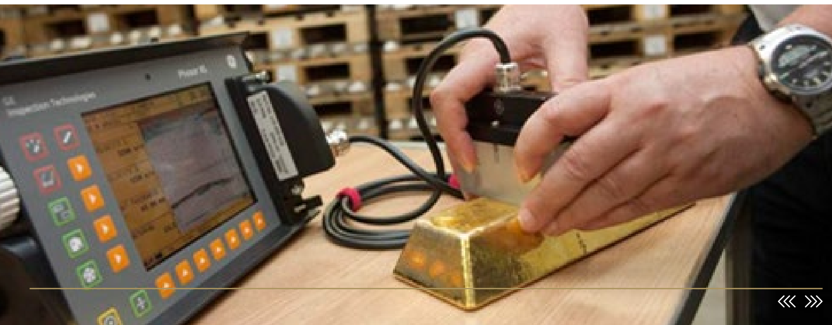
Ultrasonic testing of a gold bar
