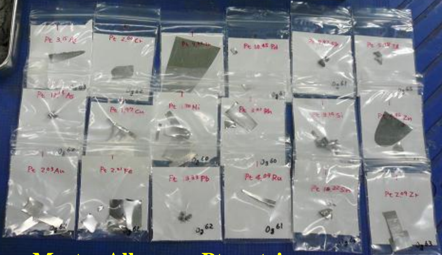
Master Alloys on Pt matrices
